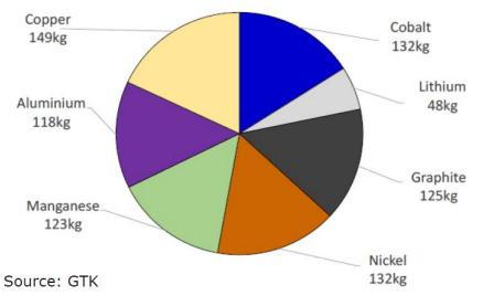
Based on 300 kWh EV (public transport) battery pack - NMC
